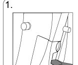
Insert a small flat blade screwdriver into the slot on the front cover.
